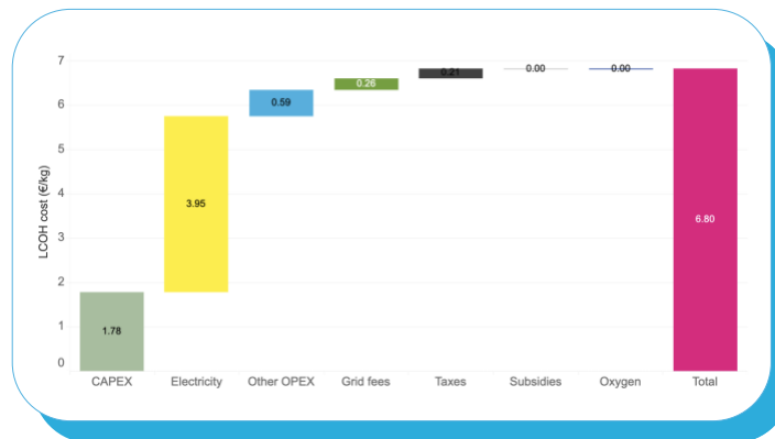
Figure 14. Use case 6 - effect of a combined electricity source on the LCOH output.
